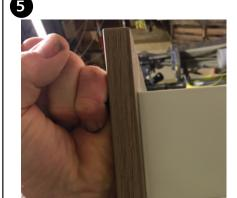
Apply light pressure with your hand or a soft face hammer until it clicks into the final locked position.
