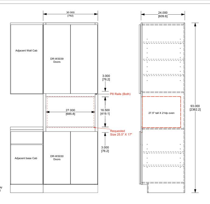
Existing design does not include overlay trim. 17" requested opening height will require on-site trimming and width exceeds requested width.
